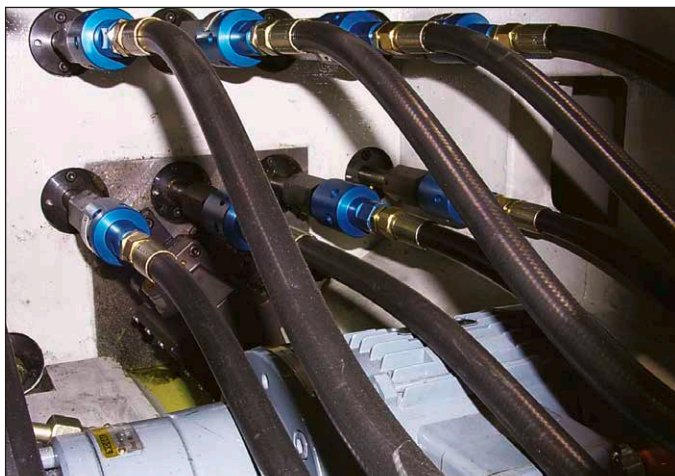
Deublin 1116 Bearing-Supported Unions on Automotive Transfer Line.
