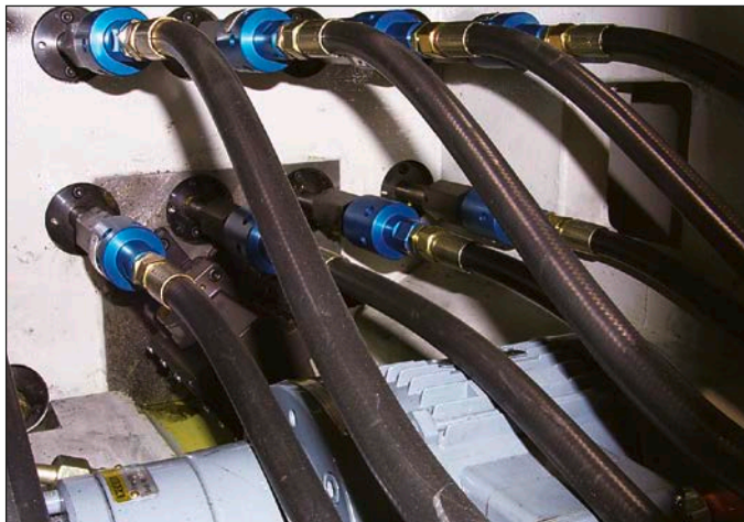
Deublin 1116 Bearing-Supported Unions on Automotive Transfer Line.
